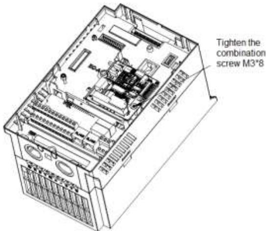
Figure 5 Installation of DeviceNet Expansion Card
