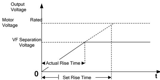
Figure 7-21 Voltage Rise Time of VF Separation
