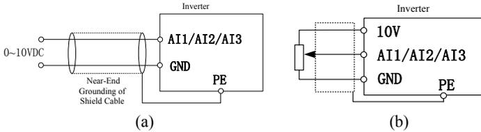
Figure 3-14 Wiring of Terminals AI1, AI2 and AI3
