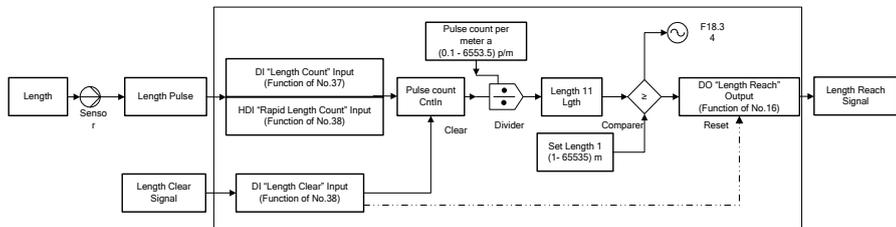
Figure 7-40 Block Diagram of Fix Length Count Function
