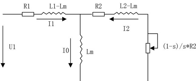
Figure 8-1 Equivalent Circuit of 3-Phase Induction Motor
