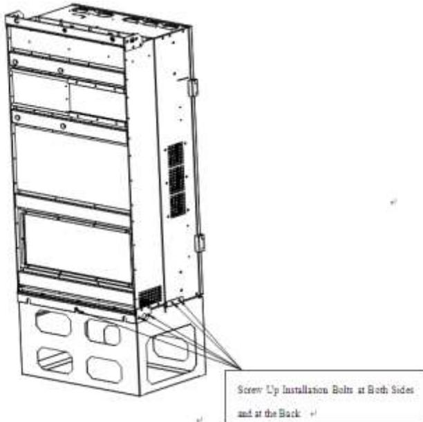
Figure 11-3 Base Installation
