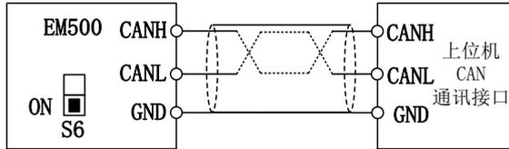
Figure 3 22 single inverter CANSinee communication wiring
