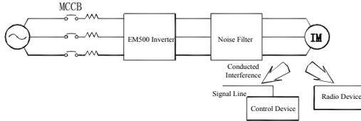
Figure 3-8 Noise Filter Installation on the Output Side
