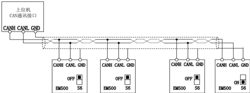
Figure 3 23 CANSinee communication wiring of several inverters
