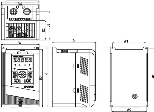
(b) Overall Dimensions of 0.75 kW – 18 kW Inverters
