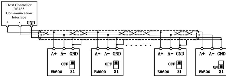
Figure 3-20 Wiring of Communication Interfaces of Multiple Inverters
