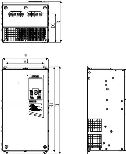
(c) Overall Dimensions of 22 kW – 75 kW Inverters
