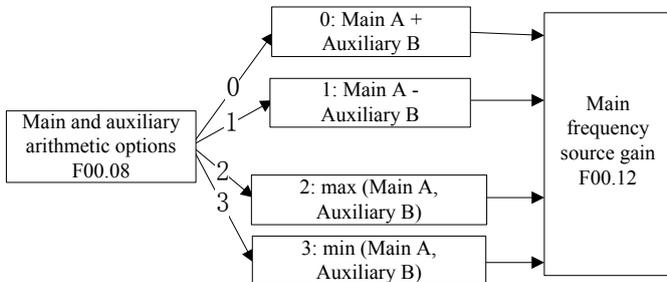
Figure 1-4 Main and Auxiliary Arithmetic Setting
