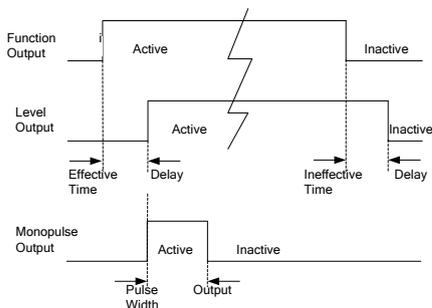
Figure 7-16 Numeric Output Terminal Level and Monopulse Output
