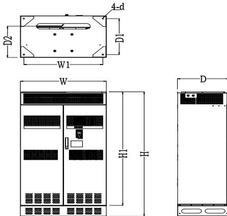
(e) Overall Dimensions of 450 kW – 560 kW Inverters
