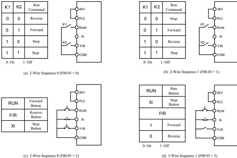
Figure 1-6 Control Logic of Terminal Control Mode
