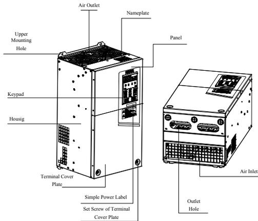
Figure 1-8 Description of Parts of EM500 Inverter (30 kW)
