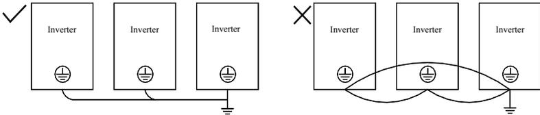
Figure 3-11 Connection Methods of Grounding Cable
