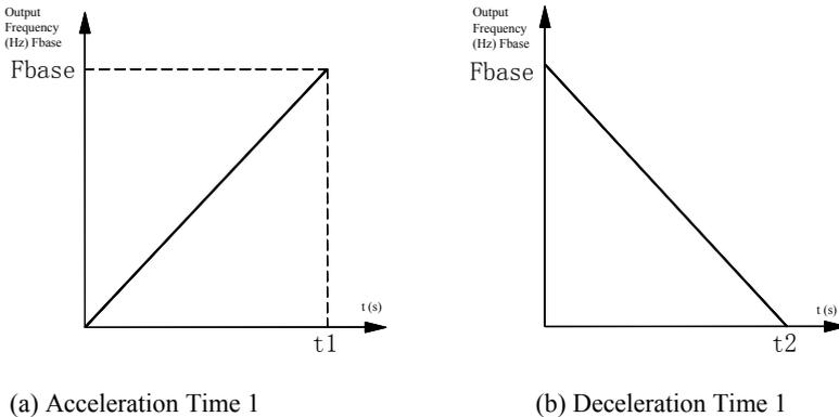
Figure 7-4 Acceleration/Deceleration Time
