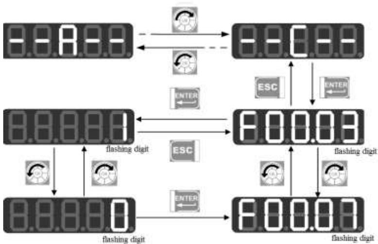
Figure 4-7 Changing Function Parameters under Non-Factory Defaults Mode
