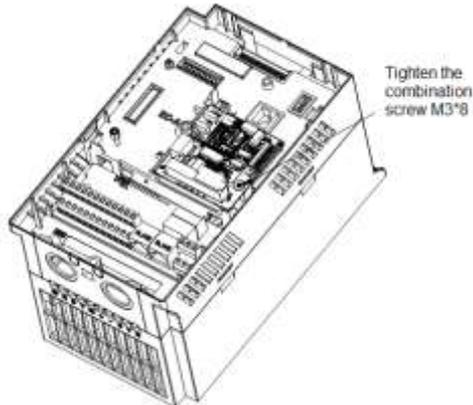
Figure 2 Installation of IO Expansion Card 3
