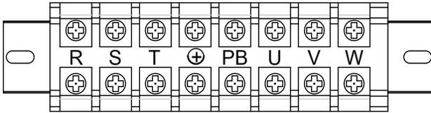
d) Main Circuit Terminal Block of Models 45 - 75 kW
