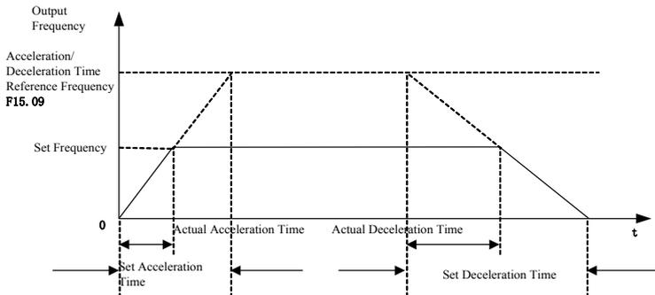
Figure 7-33 Acceleration/Deceleration Time
