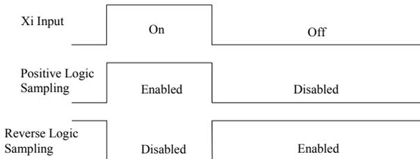
Figure 7-7 Terminal Positive and Negative Logic Sampling
