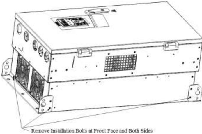
Figure 2-5 Disassemble Top and Bottom Mounting Holes
