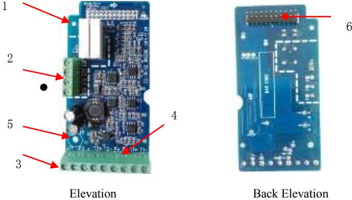
1. Output relay                      2. Relay output terminal                      3. Digital signal input interface
