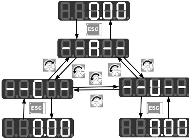
Figure 4-2 Operation Procedure of Menu Mode Selection
