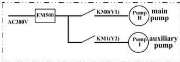
**Wiring diagram of water supply application:**
