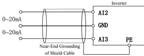
Figure 3-16 Wiring of Terminals AI2 and AI3
