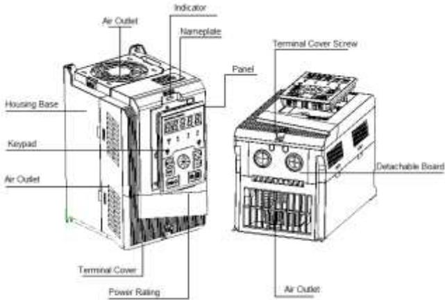
Figure 1-7 Description of Parts of EM500 Inverter (4 kW)
