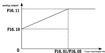
Figure 7-44 Count value and length value analog output
