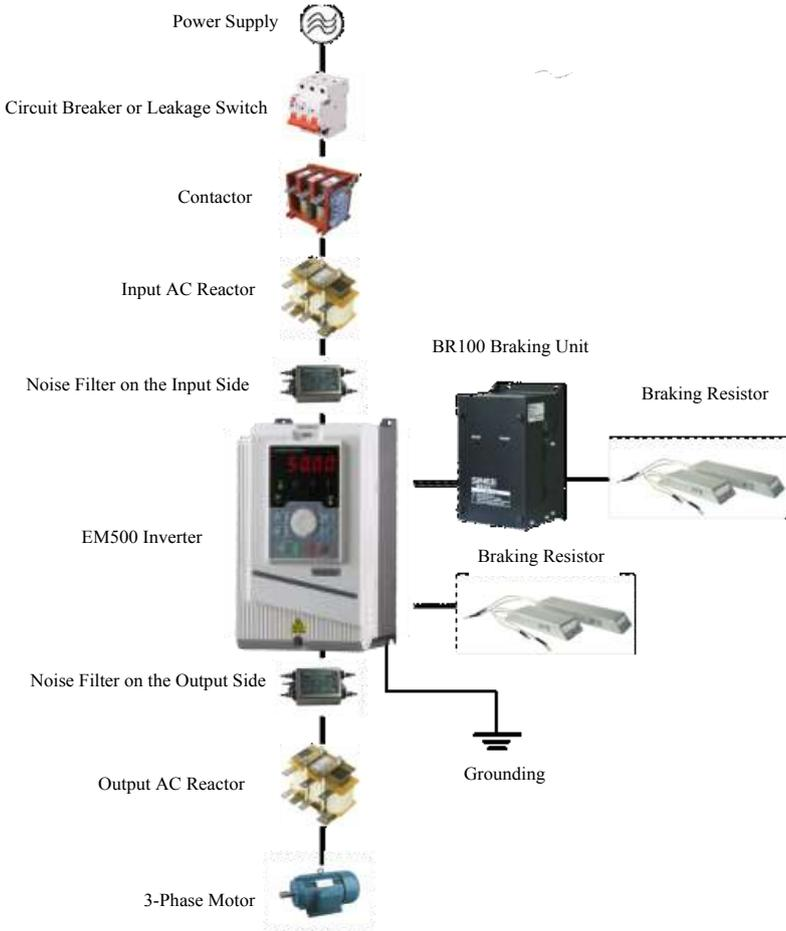
Figure 3-1 Connection of EM500 Inverter and Peripherals
