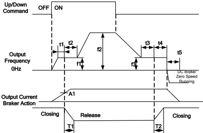
Figure 7–28 Brake Logic
