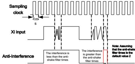
Figure 7-7 Terminal Filtering Sampling
