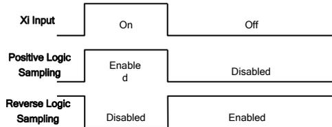
Figure 7–6 Terminal Positive and Negative Logic Sampling
