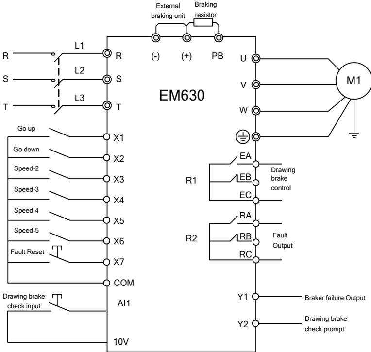
Figure 13–1 Wiring Diagram of EM630 Inverters for Hoisting Application of Tower Crane
