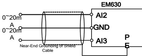
Figure 3-16 Wiring of Terminals AI2 and AI3
