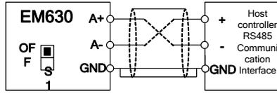
Figure 3-18 Wiring of Single Inverter Communication Interface
