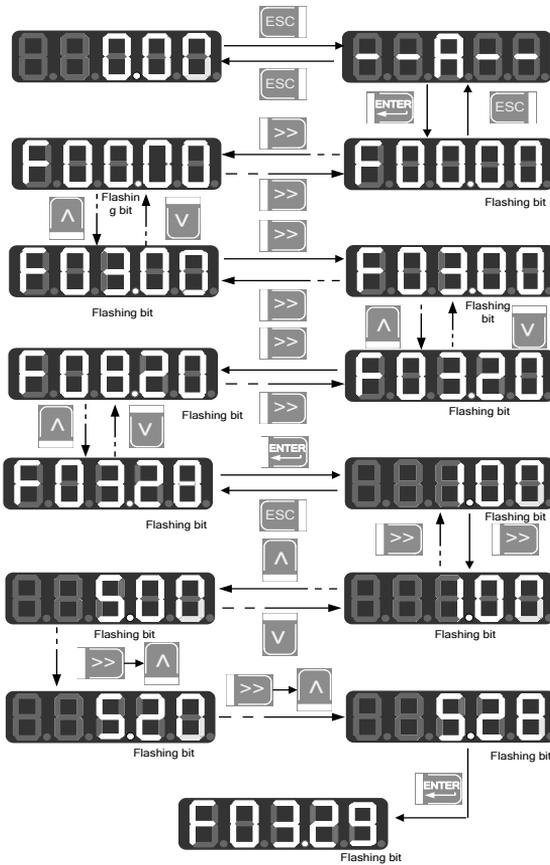
Figure 4–3 Operation Procedure from Power-on to Setting F03.28=5.28
