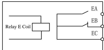
Figure 7-11 Relay Contact
