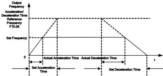
Figure 7-24 Acceleration/Deceleration Time
