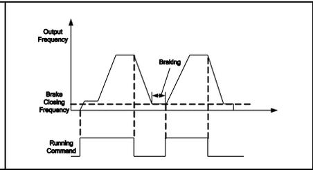
Figure 7-30 Restart Permitted at Braking
