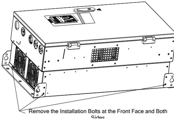
Figure 2-5 Disassemble the Top and Bottom Mounting Holes
