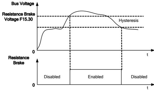
Figure 7-27 Resistance Brake
