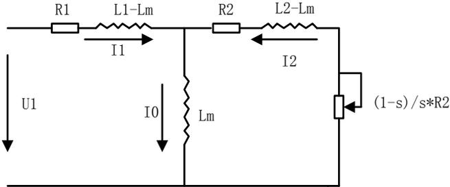
Figure 7-5 Stable Equivalent Model of Induction Motor
