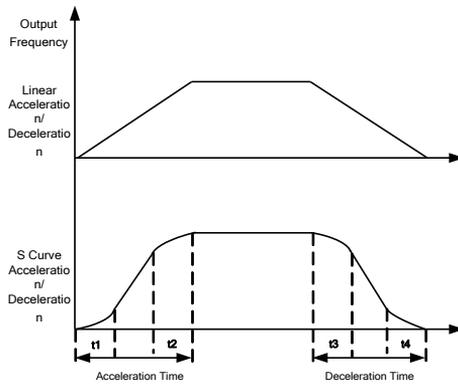
Figure 7-15 Acceleration/Deceleration Time Control
