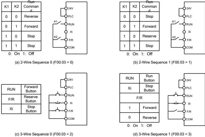
Figure 1-3 Control Logic of Terminal Control Mode
