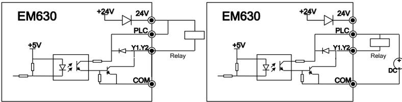
a) Internal Power Supply      b) External Power Supply
