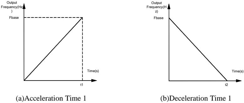
Figure 7-3 Acceleration/Deceleration Time
