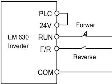
(c) F00.03=1 2-Wire Sequence Wiring Diagram
