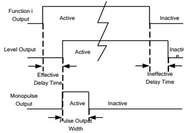
Figure 7–14 Numeric Output Terminal Level and Monopulse Output
