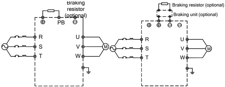
Figure 3-4 Standard Wiring of Main Circuit
