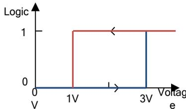
Figure 7-9 Analog Input Terminal Voltage and Present Logic Status Relationship Diagram
