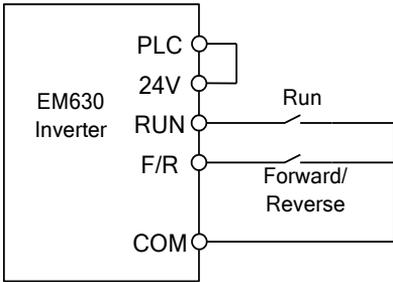
(a) F00.03=0 2-Wire Sequence Wiring Diagram
