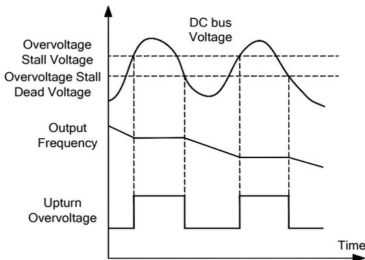
Figure 7–20 Overvoltage Stall Protection
