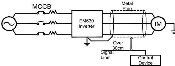
Figure 3–9 Countermeasures Against Inductive Interference
