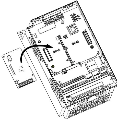
Figure 1 PG Card Installation
