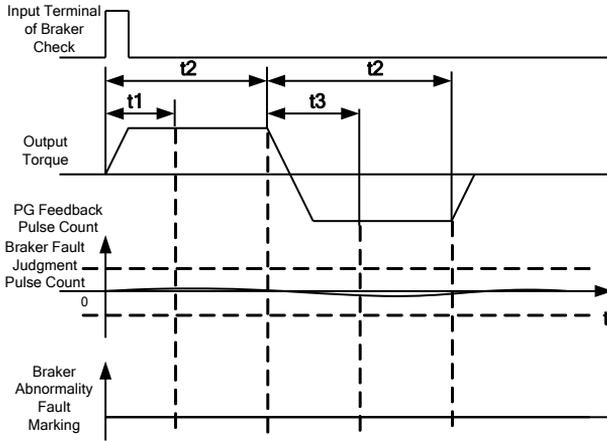
Figure 7-31 Braker Check Logic
