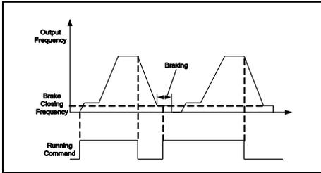
Figure 7-29 Restart Prohibited at Braking
