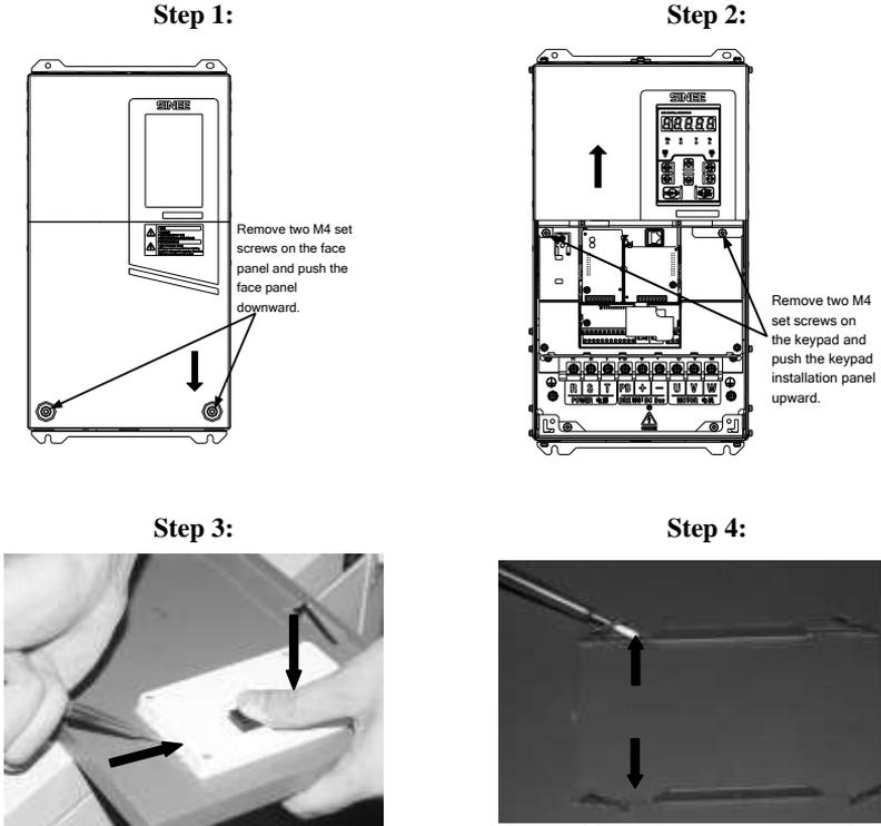
Figure 2-3 Disassemble the Keypad
