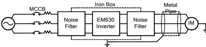
Figure 3–10 Countermeasures Against RF Interference
