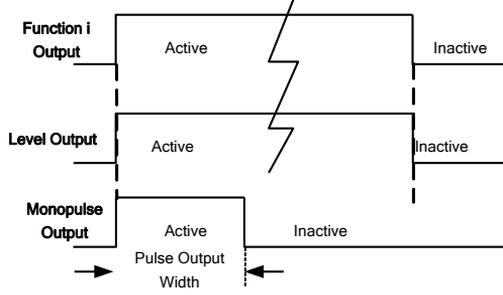
Figure 7-12 Numeric Output Terminal Level and Monopulse Output
