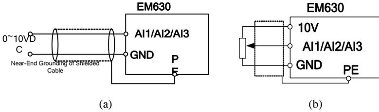
Figure 3-14 Wiring of Terminals AI1, AI2 and AI3
