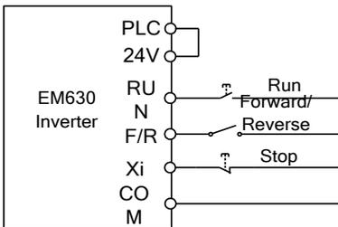
(c) F00.03=3 3-Wire Sequence Wiring Diagram
