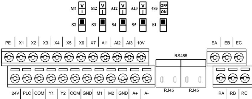
Figure 3-12 Control Circuit Terminal Block
