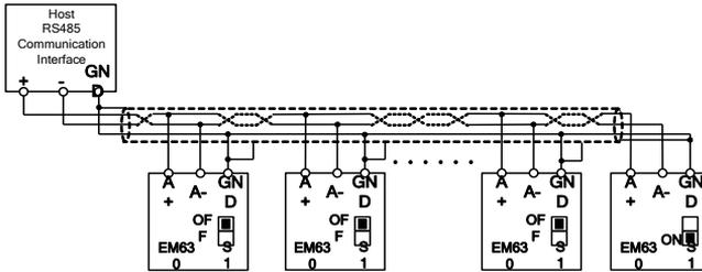
Figure 3-19 Wiring of Communication Interfaces of Multiple Inverters
