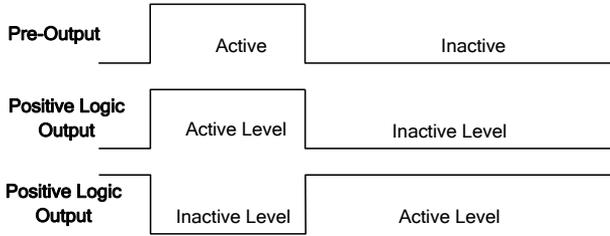
Figure 7–13 Positive and Negative Logic Output of Numeric Output Terminal
