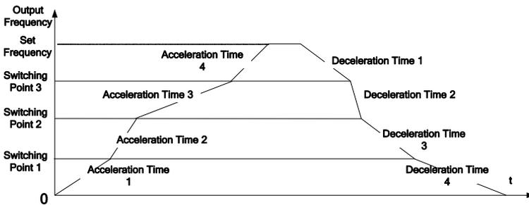
Figure 7–39 Switch between Special Acceleration and Deceleration
