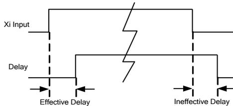
Figure 7-8 Terminal Delay Sampling
