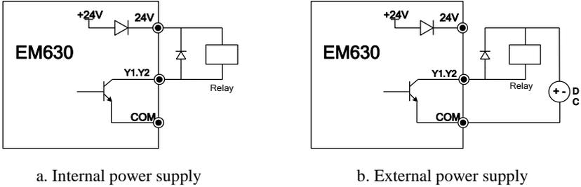
Figure 3–17 Wiring of Multi-function Output Terminal
