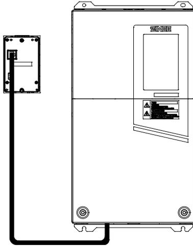
Figure 3–22 Wiring of Keypad Extension Line
