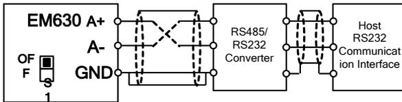
Figure 3-20 Wiring of Communication Interface
