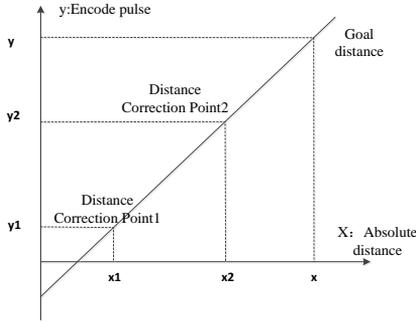
Figure 7–38 absolute distance - number of encoder pulses curve.
