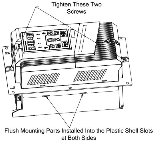
Figure 2-7 Left and Right Accessories for Flush Mounting
