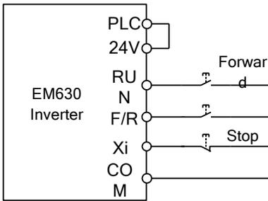
(a) F00.03=0 3-Wire Sequence Wiring Diagram
