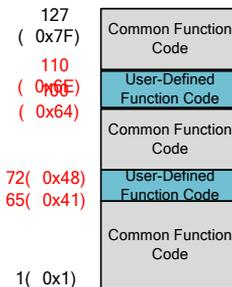
Figure 12–2 MODBUS Function Code Classification
