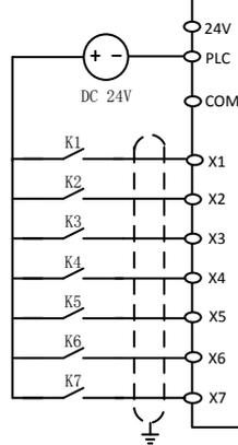
**Note:** The short-circuit bar relay output terminal wiring between 24V power supply and PLC terminal must be removed, when using an external power supply.
