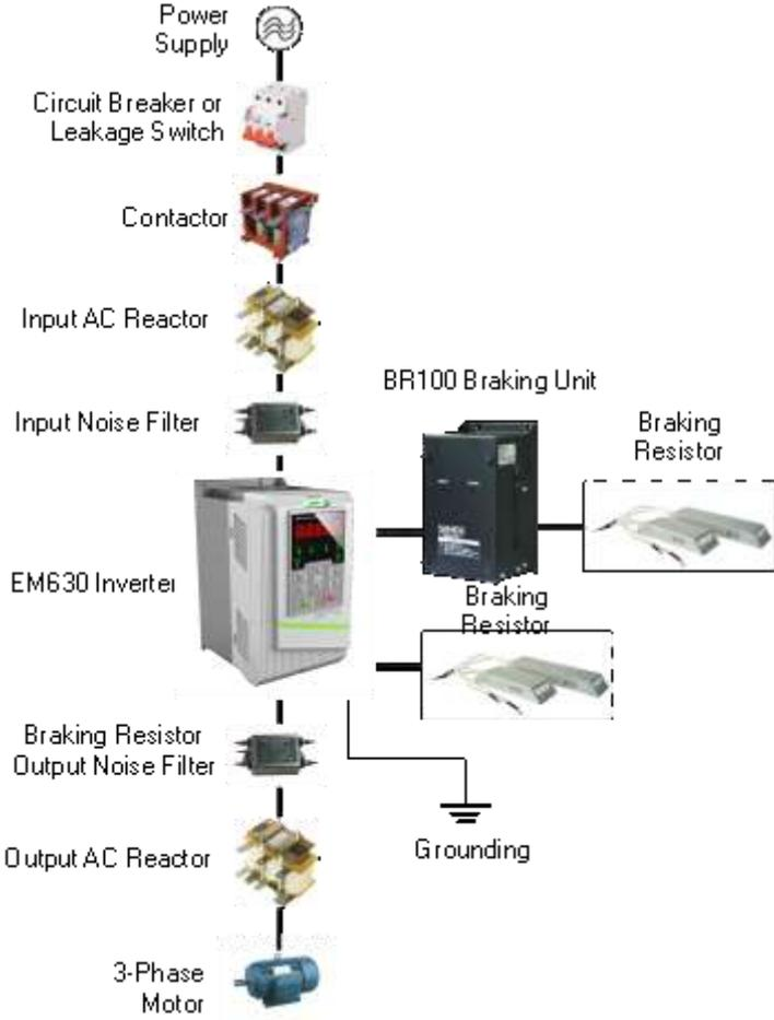
Figure 3-1 Connection of EM630 Inverter and Peripherals
