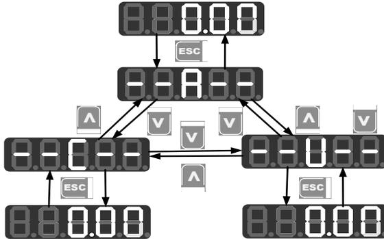
Figure 4–2 Operation Procedure of Menu Mode Selection
