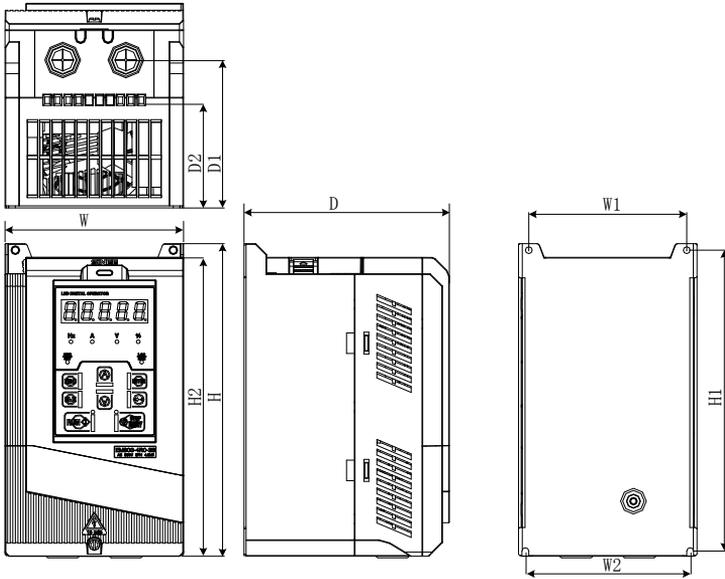
(b) Overall Dimensions of 40 kW - 18 kW Inverters
