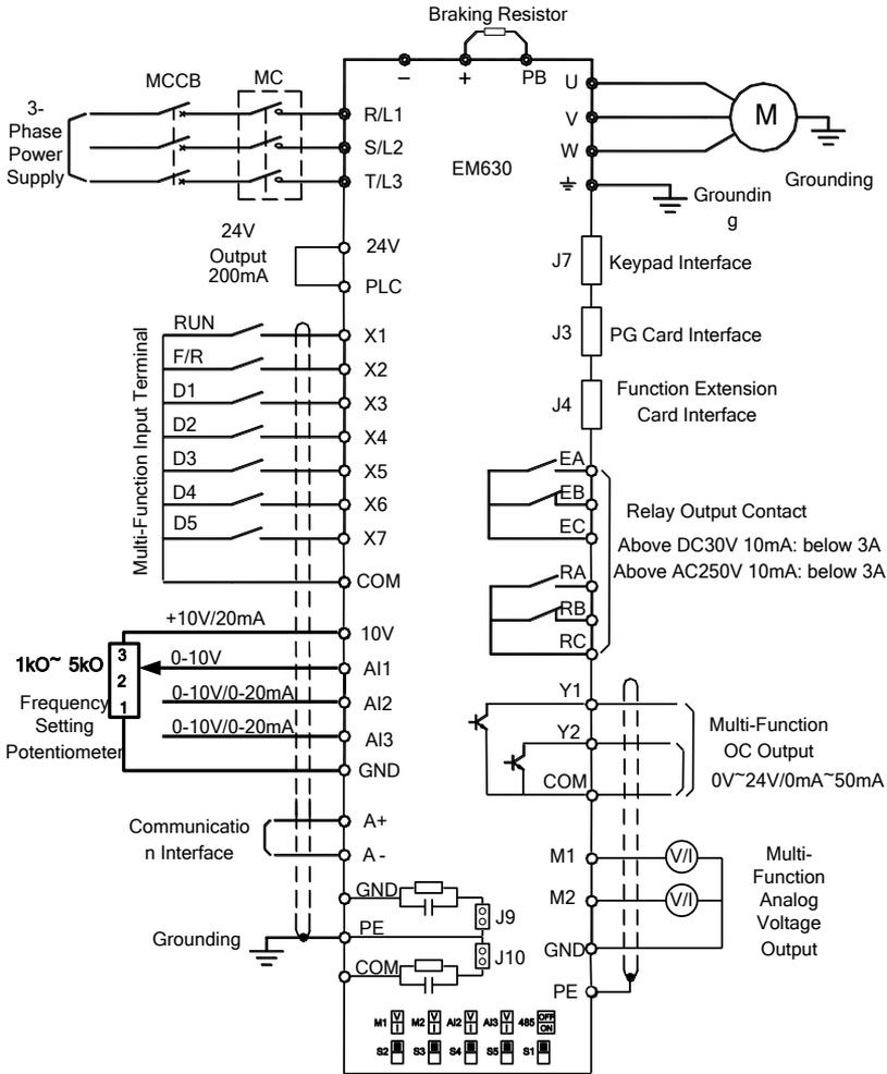
Figure 3-21 Standard Wiring of Control Circuit
