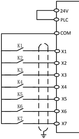
B. PNP mode with external power supply (+24Vdc)
